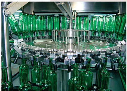
We offer you modern rinsing machines of rotary type, which turn the bottle upside-down while rinsing.
